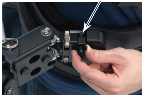
side to side: 2 turns out on top in-and-out: count threads here
