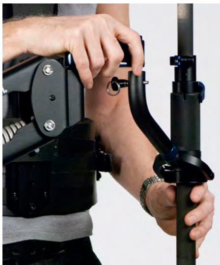
Hand positions for operating with the F-bracket.
