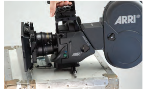
Finding the camera's fore-aft center of gravity.
