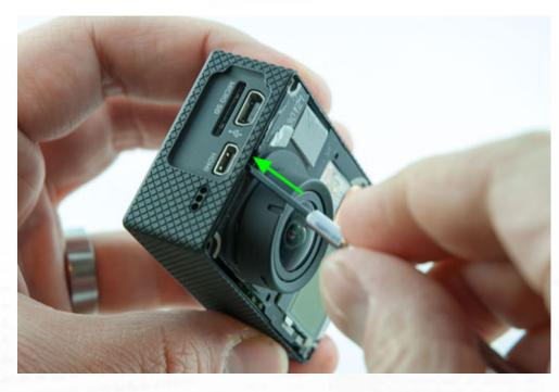
Grip the lens and work the PCB board assembly out of the housing by gently rocking the lens assembly back and forth until the internal aluminum plate and PCB board assembly is out.
