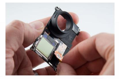
In some cases the adhesive can be stubborn and pieces of the backing may be left behind. If this is the case in your project, we recommend adding a small piece of 3M double sided tape to the affected area:
