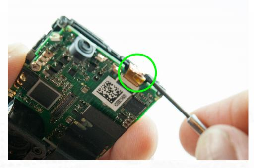
There is a small locking mechanism that grips the connector. Insert a screwdriver under the black tab and pull up to release.
