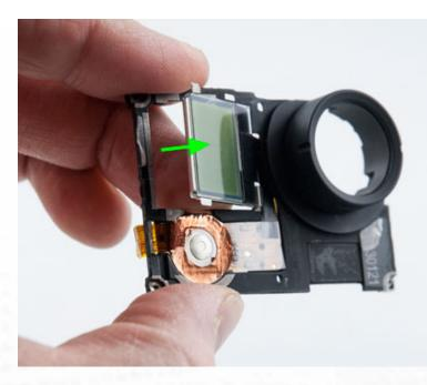
It's important to grip the LCD screen to prevent it from falling over and bending the ribbon. Pull up on the metal tape that was released earlier and gently pull the assembly free. Make sure the grey adhesive area is not stuck down when you start to pull or it may not come off properly.
