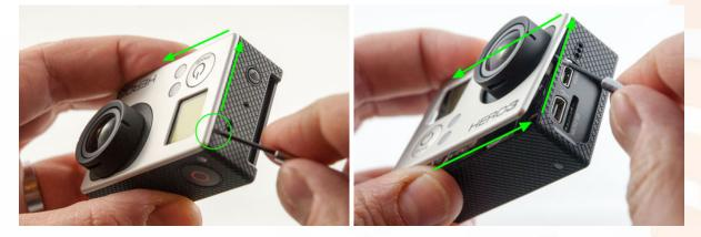
The faceplate is attached with adhesive tape and some clips. Pull the faceplate off and set it aside.
