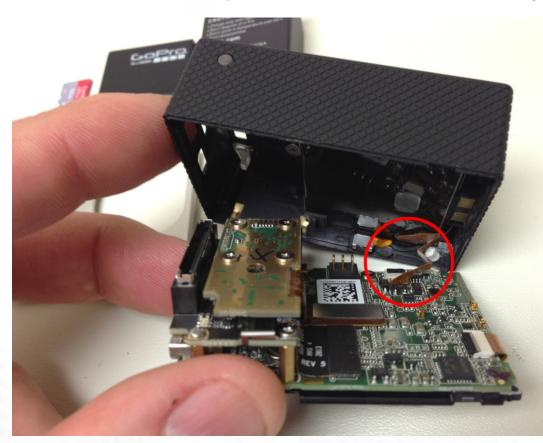
To release the ribbon pull up on the black locking mechanism, and gently pull it free.
