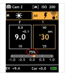
The ratio between flash and ambient light can be influenced by changing synchronization speed. This is interesting for brightening up the image with flash, or when ambient light is not desired.
