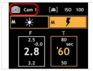
The selected user pre-set appears on the display. One of the following users can be selected: **Cam 1**, **Cam 2**, **Cam 3** or **Movie**.
