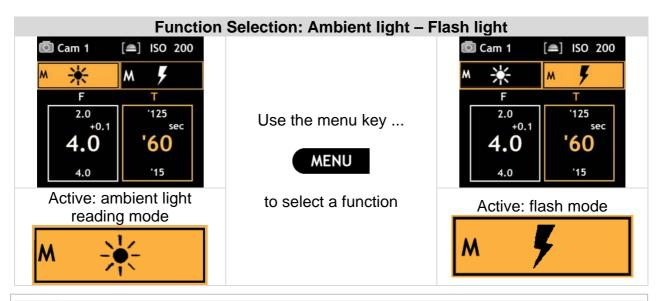
Measured f-stop increments (1 EV, 1/2 EV, 1/3 EV) can be adapted as required by the user in **Menu** – **User (Cam 1, Cam 2, Cam 3, Cine)** - **EV Steps** (see page 23).
