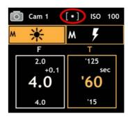
Only light reflected by the subject is measured. When this metering method is used, results are always dependent on reflection from the subject! This means, for example, that intrinsically bright subjects will be reproduced darker, and not as precisely exposed as with the incident light method.
