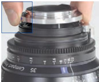
4. Tighten the torx screws using a torque of 0.25 Nm.
