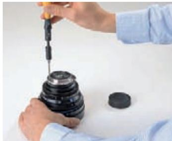
14. Recheck the flange focal distance of the lens (see section D) in combination with the camera you use.
