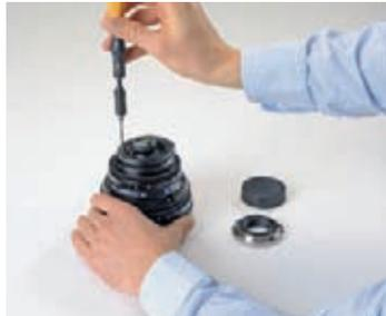
13. The next step is to place the silver EF mount on the EF adapter ring and tighten the screws using a torque of 0.25 Nm.
