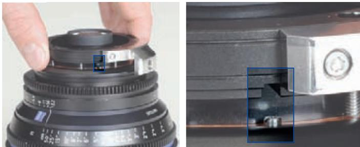
2. Place the silver EF mount on the EF adapter ring in such a way that the blue dot on the mount has the same orientation as the ZEISS logo on the lens barrel.
