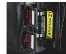
The D610's double SD card slots provide multiple options for recording and storing large files: you can write RAW and JPEG data to separate cards, copy from one card to another, or select a slot according to the remaining capacity during video shooting. The slots are UHS-I compatible, and can transfer data faster thanks to the camera's EXPEED 3 image-processing engine.
